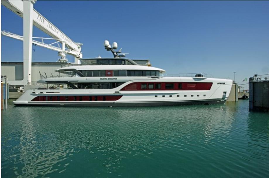
The all-aluminium *Quinta Essentia* boasts a displacement hull and hybrid drives, with naval architecture by Vripack and interior design by Michela Reverberi Studio, with an ‘elements’ interior theme: an owner’s stateroom representing earth, and the VIP water. There are four further guests cabins on the lower deck, which can be converted to two suites for a flexible cruising arrangement.
