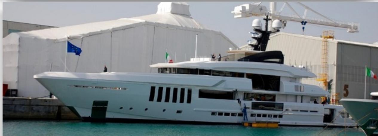
Entirely built in aluminium, **Tremenda** has a maximum speed of over **20 knots**. The shallow draft allows her to cruise in shallow waters, which makes her ideal for Caribbean cruises. This was one of the requirements the owner had in mind when he started the project.
