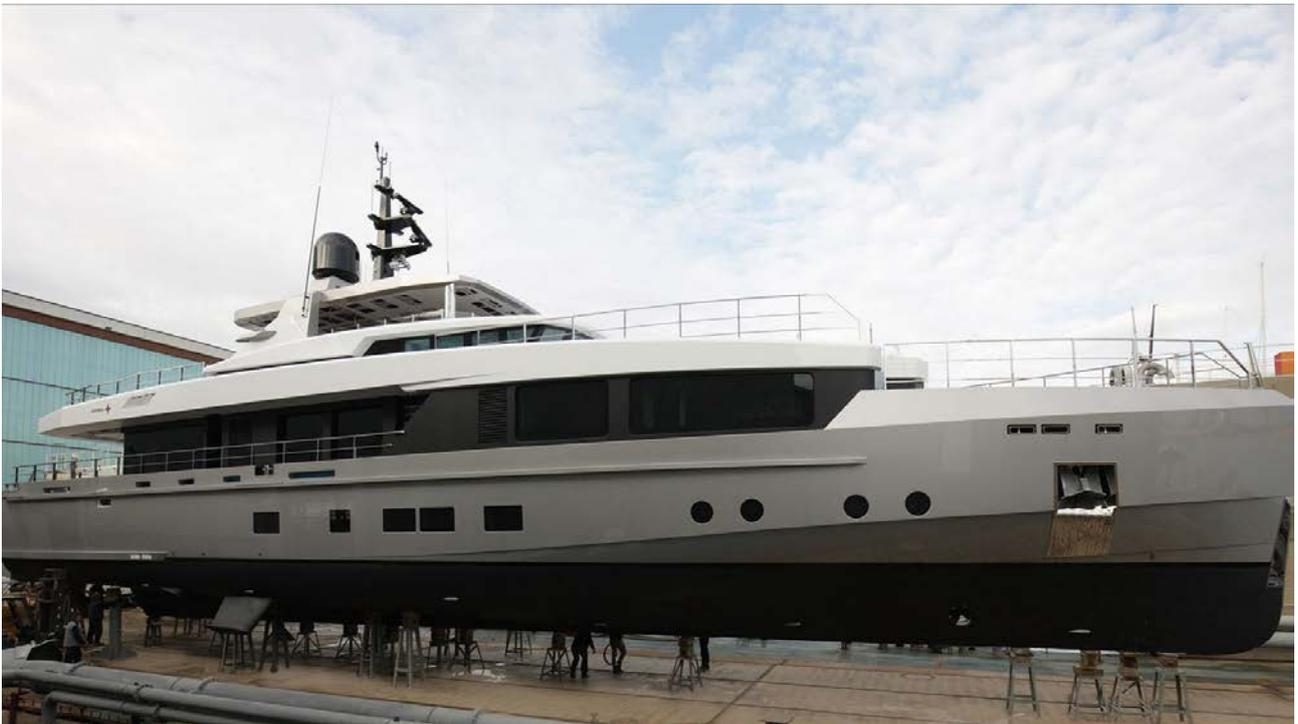
With an aluminium hull and superstructure, *Tremenda* can reach a top speed of over 20 knots. A shallow draft allows her to cruise in low depths, making her ideal for Caribbean cruises, a specific request from the owner when the project was started.
